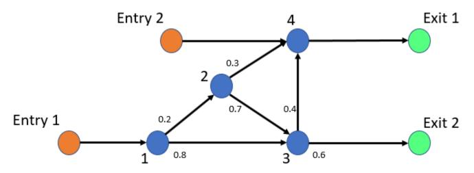
The rate of vehicle entries into the network are represented by the Poisson processes with rates 0.5 for Entry 1 and 0.15 for Entry 2. Service rates represent the time vehicles spend at each intersection, which are drawn from exponential distribution with mean 1. The arrow values are the probabilities of choosing a route for vehicles in the intersection.
