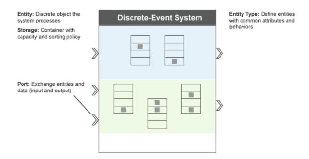
Ports enable a discrete-event System object to exchange entities and data with other blocks or model components. You can specify a variable number of input and output ports using the <code>getNumInputsImpl</code> and <code>getNumOutputsImpl</code> methods. You can also specify which ports are entity ports and the entity types for these ports. Use the <code>getEntityPortsImpl</code> method to specify these port properties.
