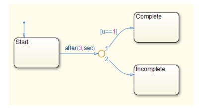
When using absolute-time temporal logic operators, observe these differences from the Stateflow environment.
