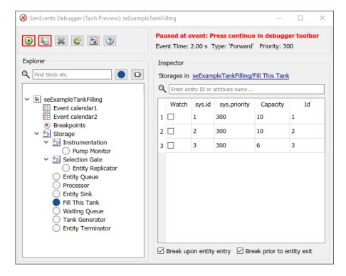
The simulation stops at the entity you opted to watch. As you continue the simulation or step through the model, the debugger stops at the various breakpoints and watchpoints that you set, letting you explore the model simulation.
