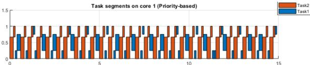
Notice that the performance of control task 2 remains unchanged. This is because the scheduler applies the priority-based policy where processing capacity is maximally assigned to high priority tasks.
