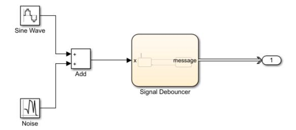
The Stateflow chart represents a simple logic that filters the signal and decides whether to send messages. If the value of the signal is greater than 0.5 for a duration greater than 0.1, then the chart sends a message that carries the signal value. If the signal value is below 0, then the chart transitions to the ReceiveSignal state. The StateflowSend component sends messages to Send Buffer 2.
