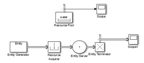
**6** Simulate the model and observe the amount of resources in use (Scope).
