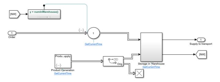
• **Transportation**: The Transportation block represents the delay, which is the duration between a product's dispatch from the warehouse and its arrival at the store. The default delay is set to two hours.
