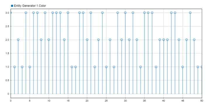
• Observe that the Diagnostic Viewer displays Color values of the third entity in each batch after batch processing.
