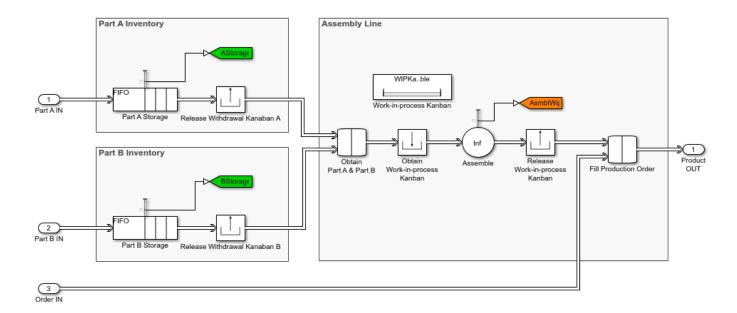
During simulation, the block labeled Obtain Withdrawal Kanban in the Part A Supplier subsystem must obtain a withdrawal kanban before a part A is transported and stored for final assembly. When a part A in storage is consumed in final assembly, the block labeled Release Withdrawal Kanban A in the Assembly Line subsystem releases the withdrawal kanban. The kanban then returns to the block labeled Obtain Withdrawal Kanban to allow replenishment of part A inventory.
