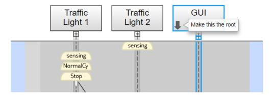
The Sequence Viewer window displays the current root lifeline path and shows its child lifelines. Any external events and messages are displayed as entering or exiting through vertical slots in the diagram gutter. When you point to a slot in the diagram gutter, a tooltip displays the name of the sending or receiving block.
