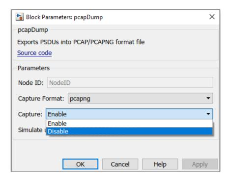
A new capture file (PCAP/PCAPNG format) is created for every node. The file name corresponds to name of the node. If name of the node is Node1, the captured file name is Node1.pcap or Node1.pcapng.
