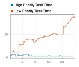
The plot displays wait time for high an low priority tasks. It can be observed that wait time of high priority tasks is significantly decreased.
