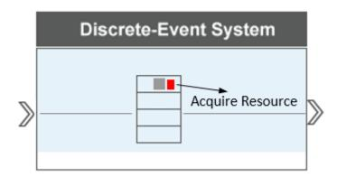
The block accepts an entity of type Part to its storage with capacity 1. The entity has an attribute Test to indicate the material from which the part is produced. Based on the value of the attribute, the entity acquires a resource from the specified Resource Pool block and departs the block to be tested.
