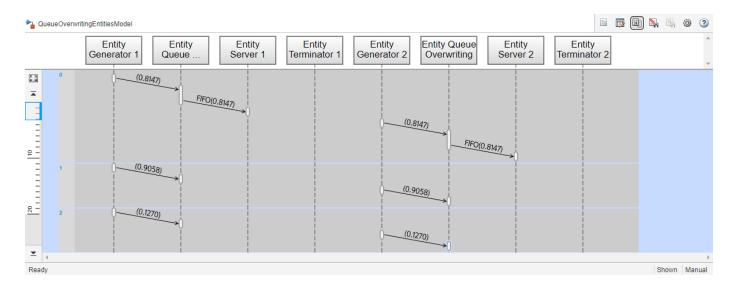
Observe that Entity Queue 1 block stops accepting new entities to its storage the time 11. However, Entity Queue 2 allows the new entity with attribute 0.9706 to storage and overwrites the oldest existing entity, which has a data value of 0.9058.
