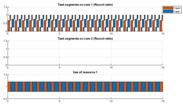
As indicated by the timing diagram, although concurrent execution is allowed with two cores, the tasks are processed in a sequential fashion. Only one core is in use. This is because a task must wait for the required resource before it can be processed.
