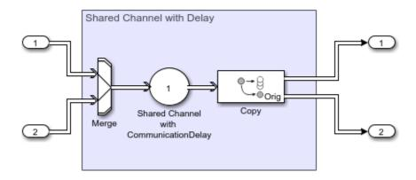
A SimEvents® Entity Input Switch block merges the message lines. In the block:
