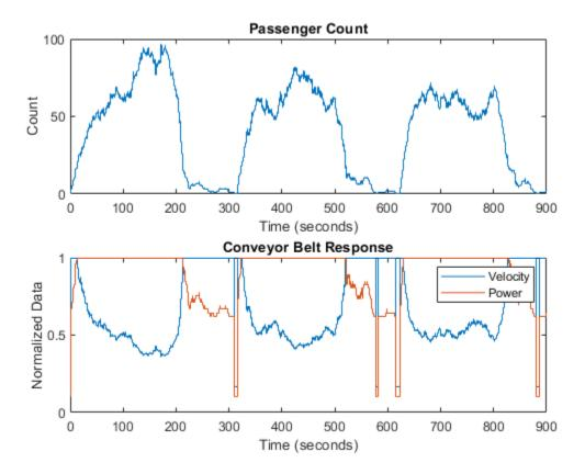
Three operation cycles are observed within a time span of 900. Each cycle has a period of 300, which aligns with the period of the arrival rate. The top plot shows the number of passengers on the conveyor belt over time, and the bottom plot shows the velocity and power of the conveyor belt. The velocity and power are normalized for better visualization.
