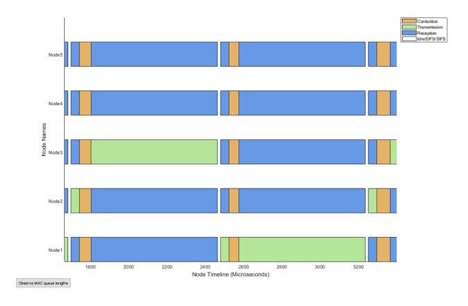
You can also observe the live state of the MAC layer transmission buffers using the 'Observe MAC queue lengths' button in the above visualization.
