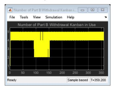
Use of withdrawal kanbans is reduced when the assembly line requests a replenishment but the part supplier fails to respond to this request in time. This leads to an analysis of the production capability of part B in the peak season of the year.
