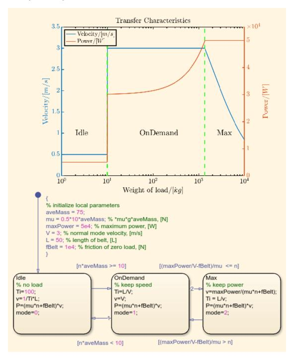
A Stateflow® chart models the dynamics of the variable speed conveyor belt. Note in the chart that the velocity and power of the belt are plotted against a logarithmic scale of the load weight. The conveyor belt has these modes:
