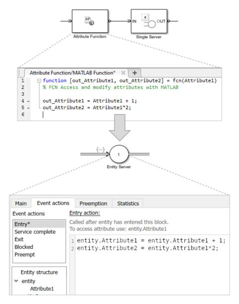
If you have longer or more complicated code, consider replacing the Attribute Function block with a Simulink Function and copying the code without modification into the Simulink Function block.
