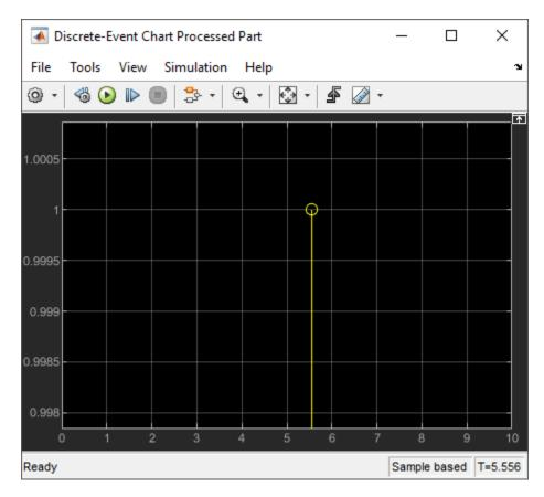
Observe that the processed Part departs the Part Generation Chart after 8 seconds, which is the sum of 5 required for part generation and quality control, 2 for the review before shipment, and 1 for the block's static scheduling.
