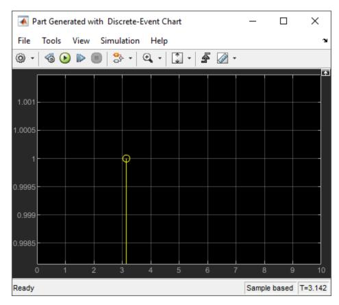
Observe that Part is generated by the Stateflow® Chart after 4 seconds. This is due to the fixed step size  $\bf 1$ , which causes the Stateflow® Chart block to wait until the next simulation step.
