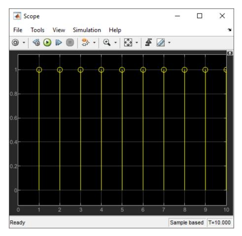
Observe the Scope block connected to the Part Generation Chart block, which displays that the parts are generated in every two seconds.
