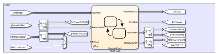
The pcapDump DES block contains two input ports, one for Tx/Rx A-MPDUs and other for Tx/Rx information.
