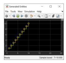
After generating 10 entities, the intergeneration time dt is set to infinity to stop generating entities. In the Entity Generator block, in the **Intergeneration time action** field, this code is used.
