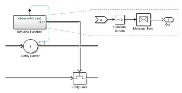
Here is an example of sending messages on trigger edges (rising, falling, or either).
