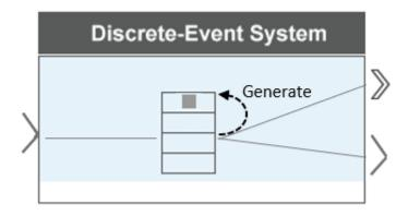
The block is defined as a custom entity generator block that generates entities with specified intergeneration periods. The generated entities carry data, and their priority values are determined by the values of the input signal.
