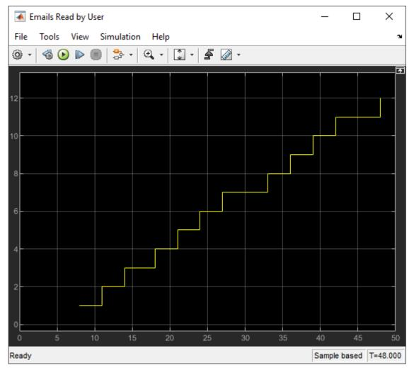
Optionally, visualize the number of extracted emails from any block in the model. For instance, in the Email Queue, select the **Number of entities extracted**, **ex** statistic and connect to a scope. Observe that six emails are extracted from the queue.
