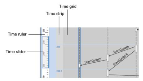
To show events in a specific simulation time range, use the scroll wheel or drag the time slider up and down the time ruler. To navigate to the beginning or end of the simulation, click the **Go to first event** or **Go to last event** buttons. To see the entire simulation duration on the time ruler, click the **Fit to view** button [3].
