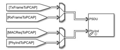
Select the capture format as pcap or pcapng. As the simulation starts, the packets exchanged between the nodes are logged into the selected capture format file.
