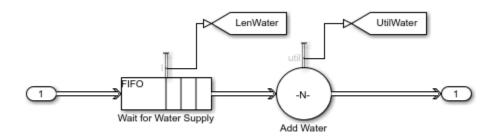
The modeled batch production process is capable of producing two types of batches: type A and type B. Although the main steps required to produce either batch are the same, the chemical process recipes are different. For example, the recipe to produce type B requires more water, so the step to add water takes more time to complete.
