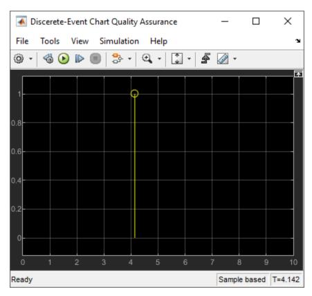
Observe the Scope block that is connected to the Quality Assurance Chart block. The block outputs the Part after 5 seconds, which is the sum of 4 seconds for the Part's generation and 1 second for its quality control as a result of fixed step size 1. This difference is based on the precise timing property of the Discrete-Event chart. For more information, see "Discrete-Event Chart Precise Timing" on page 8-6.
