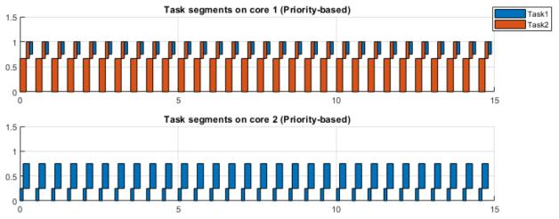
The timing diagram of the scheduler indicates that control tasks are concurrently processed by both cores, with cores having medium and balanced utilizations.
