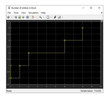
For the duration between 0 and 1, the average queue length is 0 because the size of the queue is 0. Between 1 and 2 the queue length is 1. Average queue length at time  $t_{\rm f}=2$  is calculated as follows.
