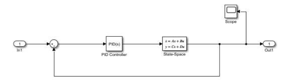
The Robot1 subsystem is designed to track a reference signal from the In1 block, which is the out signal from the Discrete-Event Chart block. The system compares the input value with the output from the State-Space block and the difference between signals is fed to the PID Controller block.
