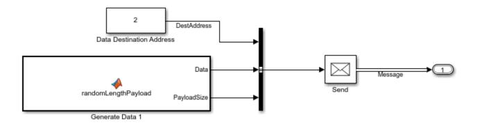
Each computer generates data with a different rate. You can change the data generation rate from the MATLAB Function block's sample time.
