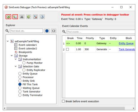
2 To inspect the attributes of an entity, click the **Fill This Tank** storage element in the **Explorer** pane.
