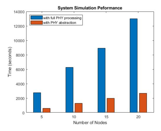
This example explained the physical layer abstraction and demonstrated a 10-node WLAN network with abstracted PHY. This example shows that a network simulation with abstracted PHY is faster and more scalable compared to using full PHY processing.
