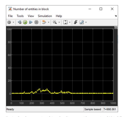
To visualize the proportion of time that the queue with a capacity of 10 is full, the statistic signal is further processed and compared to zero.
