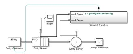
A subset of the blocks in SimEvents library provides statistics output for run-time control. When you create simulations that use statistical signals to control the dynamics, you access the current statistical values at key times throughout the simulation, not just at the end of the simulation.
