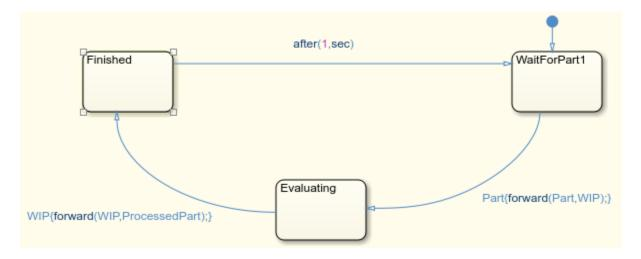
Similarly, the Quality Assurance is modeled by a Discrete-Event Chart while the Quality Assurance Chart is modeled by a Stateflow® Chart block. Both blocks contain the same state transition logic including three states, WaitForPart, Evaluating, and Finished.
