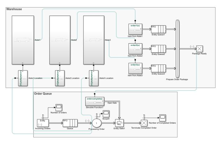
In this model, an online order for multiple items arrives at the Order Queue component. The locations of the ordered items are communicated from the Processing Order block to the autonomous robots in the Warehouse component. Three robots are assigned to three aisles. A robot picks up an item from its aisle location and returns it to its initial location for delivery. An order can have one, two, or three
