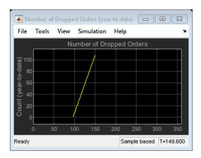
**Step 2:** Comparing the demand in peak season with product supply indicates the assembly line does not provide sufficient production capability. According to the scope labeled Product Demand (see the figure above), 10 products are needed daily between day 90 and day 150. In contrast, as illustrated by the scope labeled Number of Products in Final Assembly (see the figure below), in the same period of time, only about 5 are in production every day - much less than the quantity in demand.
