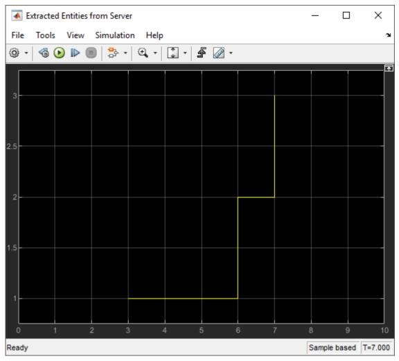
6 Observe that 3 found entities are extracted from the Entity Server block and terminated in the Entity Terminator1 block.
