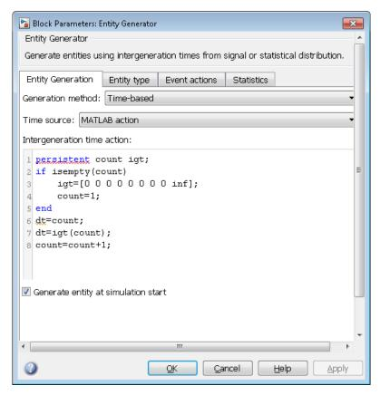
In the **Events action** tab, randomize the entity attribute. Select the **Generate** event action and, in the **Generate action** field, enter the MATLAB code:
