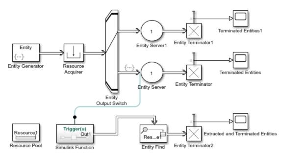
To open the model, see Trigger Entity Find Example.
